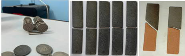
Fig. 4. Samples of ceramic membranes printed by the SLS method
