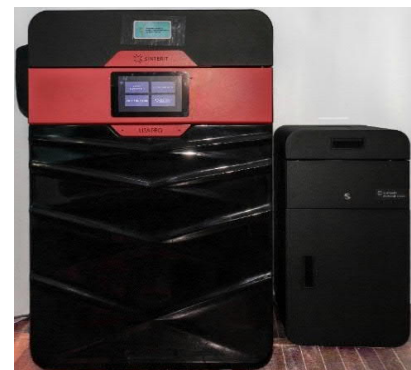
Fig. 3. Lisa PRO 3D-printer and powder mixing station
