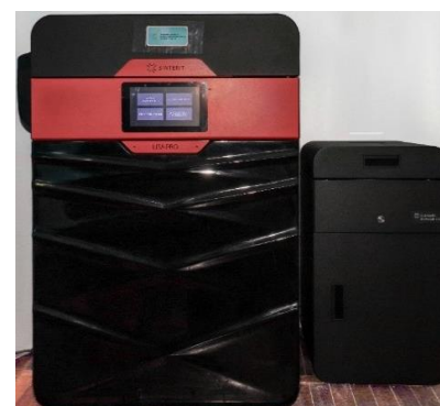
Fig. 3. Lisa PRO 3D-printer and powder mixing station
