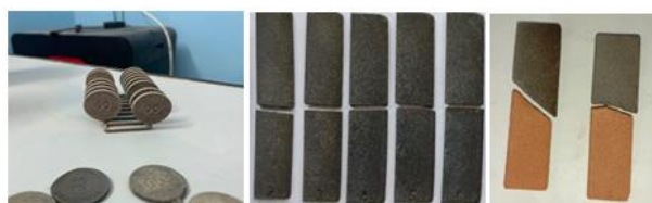
Fig. 4. Samples of ceramic membranes printed by the SLS method
