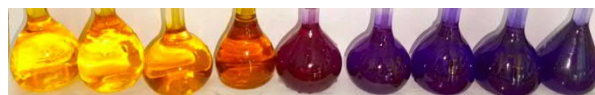
Fig 2. Color changes of chromazurol S in the presence of different concentrations of zirconyl ions
