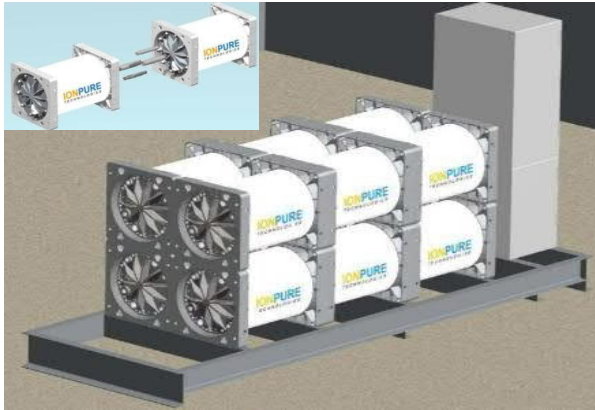
Figure 2. System of modules connected in a line using connecting tubes (Al-Rawajfeh, 2014)
