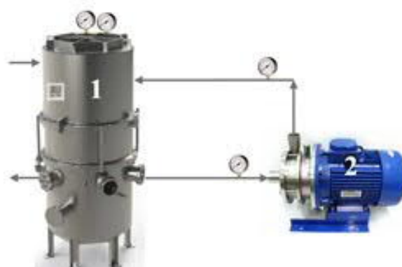
Fig. 1. Experimental stand: 1 - storage tank; 2 - RPA
