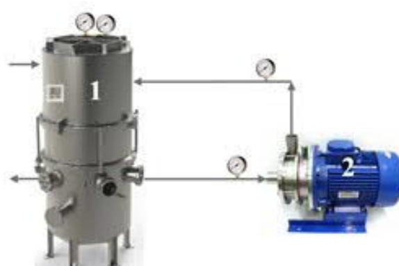
Fig. 1. Experimental stand: 1 - storage tank; 2 - RPA
