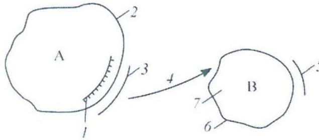
**Fig. 4.** Scheme of oxygen transfer from gas bubbles to microorganisms: A – an air bubble, B – a cluster of microorganisms, 1 – diffuse boundary layer from the gas side, 2 – interface, 3 – diffuse boundary layer from the liquid side, 4 – transfer of oxygen from gas bubbles to microorganisms, 5 – diffuse boundary layer from the liquid side to microorganisms, 6 – transfer of oxygen inside the cells, 7 – reaction between oxygen molecules and enzymes
