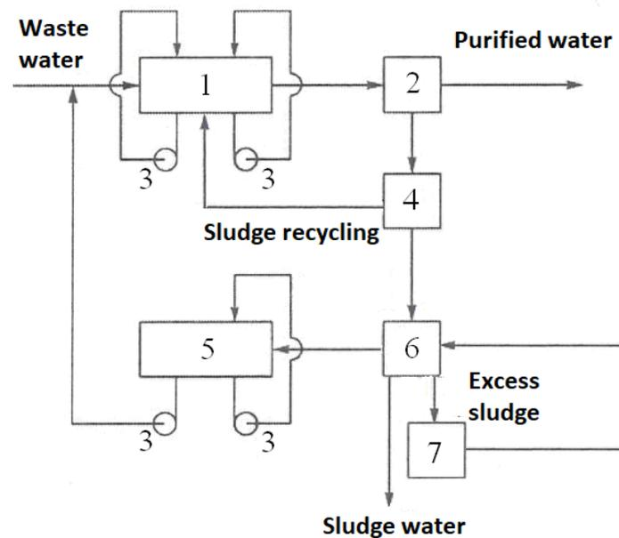
**Fig.3.** Scheme of biological wastewater treatment using AORT: 1 – aeration tank, 2 – sedimentation tank, 3 – rotor-type aerator-oxidizer, 4 – collector, 5 – regenerator, 6 – sludge compactor, 7 – sludge platform
