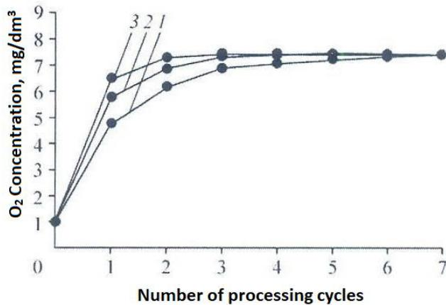
**Fig.6.** Dependence of dissolved oxygen concentration on the number of processing cycles at different pulsation frequencies: 1 – 2.0; 2 – 2.4; 3 – 2.8 kHz;  $n = 47.75$  rpm; the inter-cylinder gap is  $150 \mu\text{m}$
