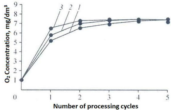
**Fig.7.** Dependence of dissolved oxygen concentration on the number of treatment cycles at different flow shear rates: 1 –  $57 \cdot 10^3 \text{ c}^{-1}$ ; 2 –  $85.5 \cdot 10^3 \text{ c}^{-1}$ ; 3 –  $114 \cdot 10^3 \text{ c}^{-1}$ ;  $n = 47.75$  rpm; number of slots – 60
