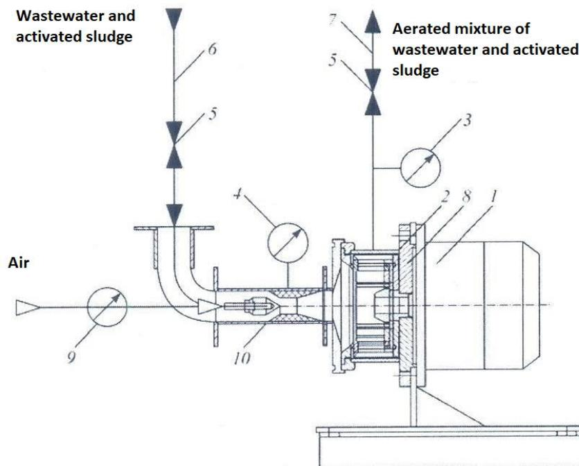
**Fig.1.** Scheme of a rotary-type aerator-oxidizer: 1 – electric motor, 2 – rotary-pulsation unit, 3 – manometer for measuring the pressure at the outlet of the RPU, 4 – vacuum meter for measuring the discharge in the inlet pipe, 5 – two-way pipe, 6 – receiving pipeline, 7 – discharge pipeline, 8 – housing of the rotor-pulsation device, 9 – rotameter, 10 – ejector unit
