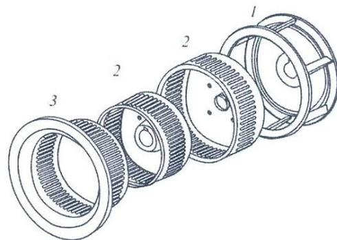
**Fig.2.** Working bodies of the rotary-pulsation unit: 1 – centrifugal pump impeller, 2 – rotor, 3 – stator
