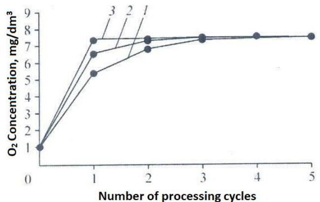
**Fig.5.** Dependence of the concentration of dissolved oxygen on the number of processing cycles at the angular speed of rotation of the RA: 1 – 38.2; 2 – 47.75; 3 – 52.52 rpm; number of slots – 60; the inter-cylinder gap is 150 μm
